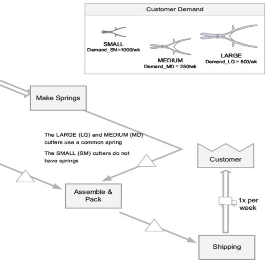
The plant is operational for 16 hours each day with two 8-hour shifts, 5 days a week, providing each shift with a 30-minute lunch break, two 15-minute breaks, and a 10-minute cleanup at the end of each day.
